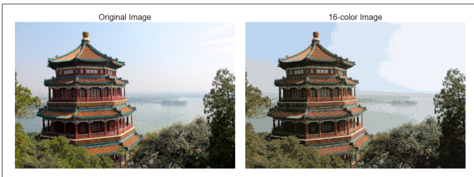
Figure 5-123. A comparison of the full-color image (left) and the 16-color image (right)
